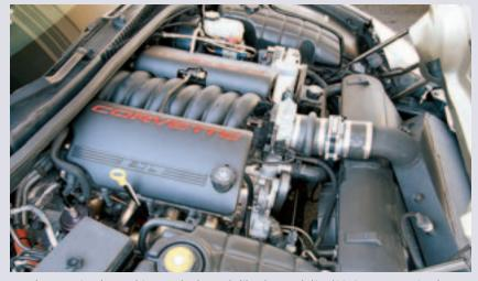
For the untrained eye, this may look much like the stock '97-'03 Corvette engine bay. But, in fact, this LS1 engine is outfitted with twin ball-bearing turbochargers netting close to 1,100 hp.
